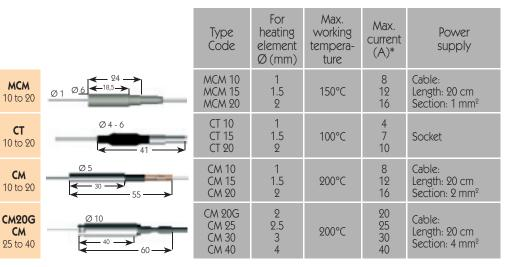
\*) These values are given for a mounting on a ZEZ type heating element. For the types 1Nc and 1Hc, divide the values respectively by 4 and 6.
